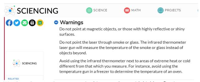
Warnings: Do not point at magnetic objects, or those with highly reflective or shiny surfaces. Do not point the laser through smoke or glass. The infrared thermometer laser gun will measure the temperature of the smoke or glass instead of objects beyond. Avoid using the infrared thermometer next to areas of extreme heat or cold different from that which you measure. For instance, avoid using the temperature gun in a freezer to determine the temperature of an oven.
